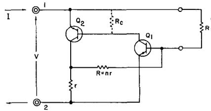
Fig. 1. The configuration of the simple negative impedance circuit.
